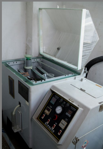
▲ Salt spray test 24H Acid, 48H neutral
