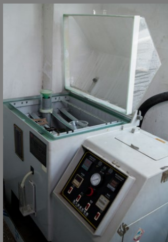
▲ Salt spray test 24H Acid, 48H neutral
