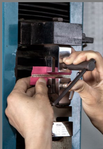
▲ Transverse tensile test of zipper
